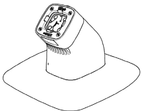
The TableTop with Base can be mounted directly to any surface using four (4) M6 screws (not included) with appropriate length for your surface. Use the mounting pattern to the right for proper alignment.
