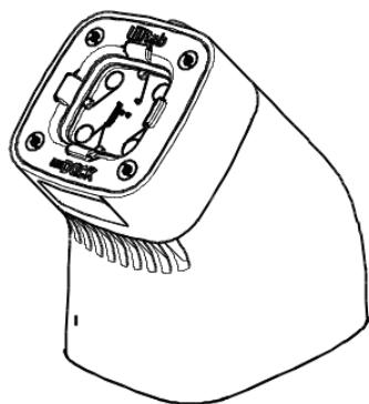
The TableTop can be mounted directly to any surface using four (4) M4 screws (not included) with appropriate length for your surface. Use the mounting pattern to the right for proper alignment.
