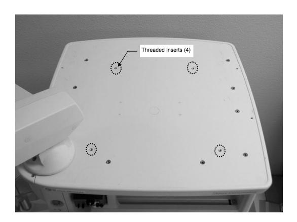
2. Align four (4) mounting holes in Top Plate with corresponding threaded inserts in top of machine. Fasten Top Plate to top of machine with four (4) M5 x 12mm FHMS.
