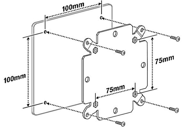
Displays with a 100 x 100mm mounting pattern require attachment of the 75 to 100mm VESA Mounting Adapter to the display.
