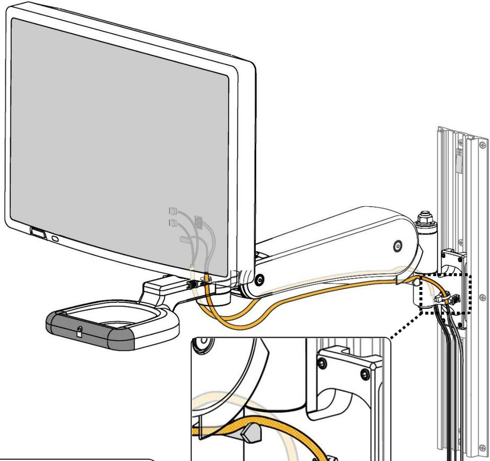
**Position cable tie heads flush against the arm while tightening.**
