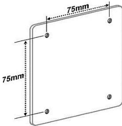
Displays with a 75 x 75mm mounting pattern will be fastened directly to the VESA mounting plate on the Arm.
