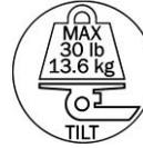
Maximum weight for mounting plate with tilt function.
