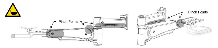
• Due to risk of personal injury or damage to the arm, the arm housing must never be disassembled by non-GCX personnel. Failure to comply will void the warranty.
