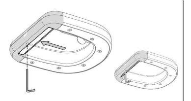
Move the arm to a level horizontal position and use a 5/32" hex wrench to increase (+) or decrease (-) the counterbalance setting. Counterbalance is correctly set when the arm can be moved up or down with minimal force. A small amount of residual float up or down is okay and may be set per user preference. Arms with minimum payloads may encounter up to 4 lb (1.8 kg) of upward float even with the counter balance setting adjusted to the minimum; this is a normal condition.
