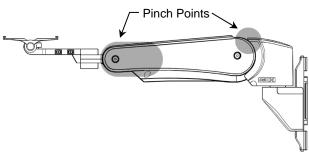
• Remove the device only when the arm is at the highest position. Due to the counterbalance function, the arm will naturally rise to the highest position when weight is removed. This can happen suddenly if the weight is removed at any height other than the highest point.
