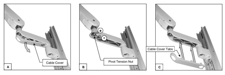
6.6 Rear Pivot Tension Adjustment – To adjust the tension at the rear Pivot Point (closest to channel), tighten (+) or loosen (-) the Pivot Tension Nut with a 3/4" or a 19 mm socket wrench until desired tension is achieved. Do not remove the Pivot Tension Nut.
