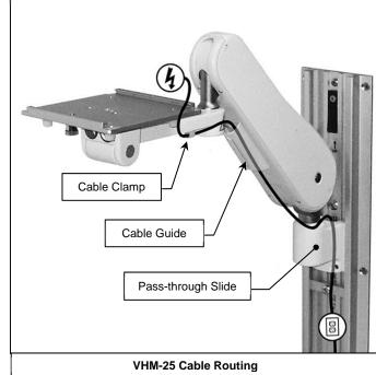
7.1.3 Cable Clamps (1/4" and 3/16" diameters) are supplied in order to secure device cables to the underside of the front extension. To install, press Cable Clamp onto cable (Fig. A) and secure with (1) 8-32 x 5/16" PHMS to any of the (4) Cable Clamp Mounting Holes as shown below. Do not use the Accessory Mounting Holes for Cable Clamps. The Arm is designed to accommodate (4) Cable Clamps, however extra Cable Clamps are provided.
