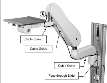
7.2.2 An open cavity beneath the extension with a removable Cable Cover manages cables going between the Arm and the pass-through slide. To install cables, remove Cable Cover by inserting finger into the front of the Cable Cover and pulling down (Fig. B). Push Cables into Cable Cover access holes as shown (Fig. C). Reinstall Cable Cover by pushing it up into the Arm until it snaps into place (Fig. D).
