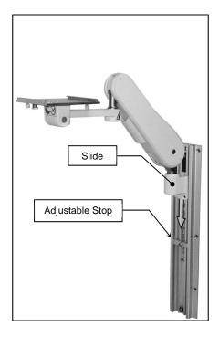
**4.3** Using a 1/8" hex wrench (supplied), tighten (CW) the (2) set screws in the Slide to secure position of Arm.
