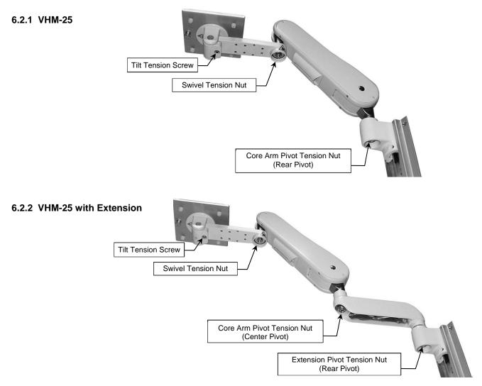
**6.3** Tilt Tension Adjustment – Using a 5/32 hex wrench, tighten (+) or loosen (-) the Tilt Tension Adjustment Screw until desired Tilt Tension is achieved. Adjustment range is approximately 1/2 turn total. Do not remove or over-torque the Adjustment Screw.
