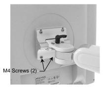
**"Slide-in" Type:** Pull the Plunger at the front of the Mounting Plate. Slide the instrument Mounting Adapter into the Mounting Plate until the Plunger snaps into the clearance hole in the Adapter. Tighten the Nylon screws on the rear or underside of the Plate.
