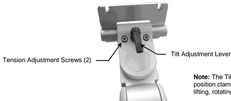
**Note:** The Tilt Adjustment Lever is a multi-position clamping lever that operates by lifting, rotating, and releasing the handle.
