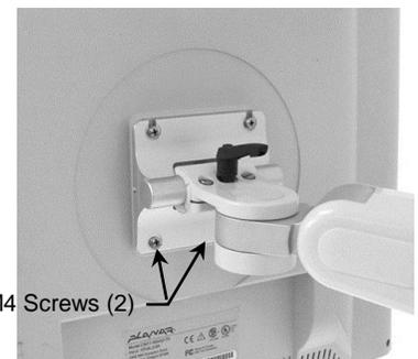
**“Slide-on” Type:** Pull the Plunger at the front of the Mounting Plate. Slide the instrument Mounting Adapter into the Mounting Plate until the Plunger snaps into the clearance hole in the Adapter. Tighten the Nylon screws on the rear or underside of the Plate.
