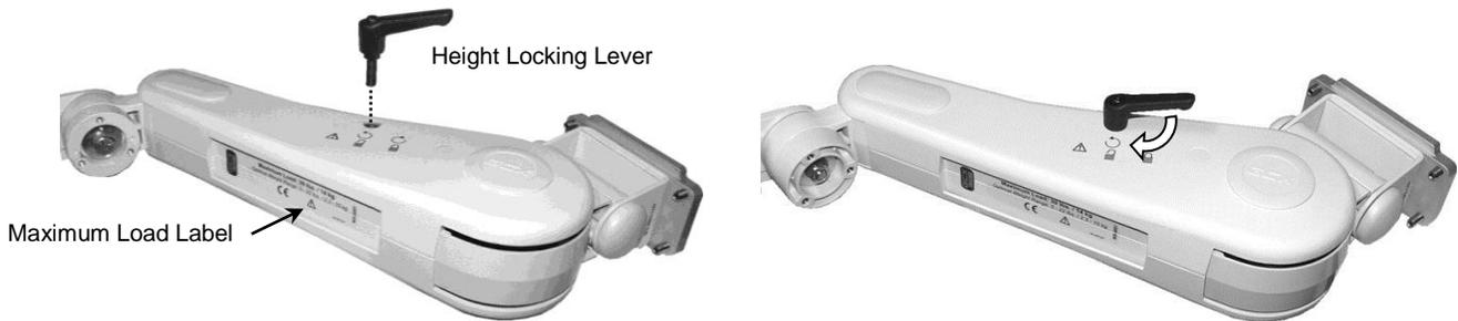
**Note:** The Height Locking Lever is a multi-position clamping lever that operates by lifting, rotating, and releasing the handle.
