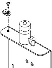
2. Position cable or wire through cable clip and secure cable clip back to Camera Mount Bracket with 6-32 x 3/16" PHMS using a Phillips screwdriver.
