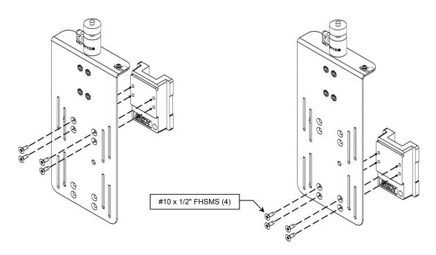
2. Guide Camera Mount Bracket to desired height in channel. (For VHRC applications, channel cover will need to be removed.)
