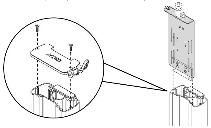
3. Once Camera Mount Bracket is at desired height, tighten two (2) set screws with 1/8" Hex Wrench (provided). Replace VHRC Top Plate once Camera Mount Bracket is secured in place.
