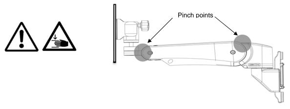
• Remove the Device only when the Arm is at the highest position. Due to the counter balance function, the Arm will naturally rise to the highest position when weight is removed. This can happen suddenly if the weight is removed at any height other than the highest point.
