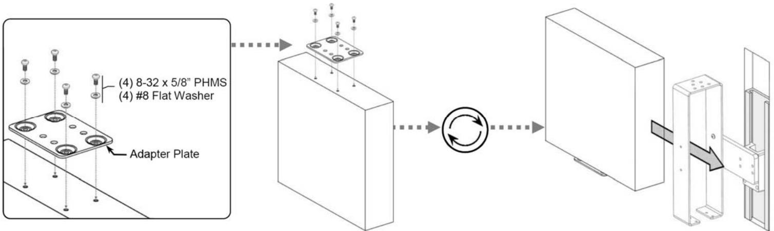
2. Align the (4) mounting holes on the Flush Mount with the (4) threaded mounting holes on the adapter plate. Using a Phillips screwdriver, secure the module housing with (4) 8-32 x 1/4" FHMS as shown below.
