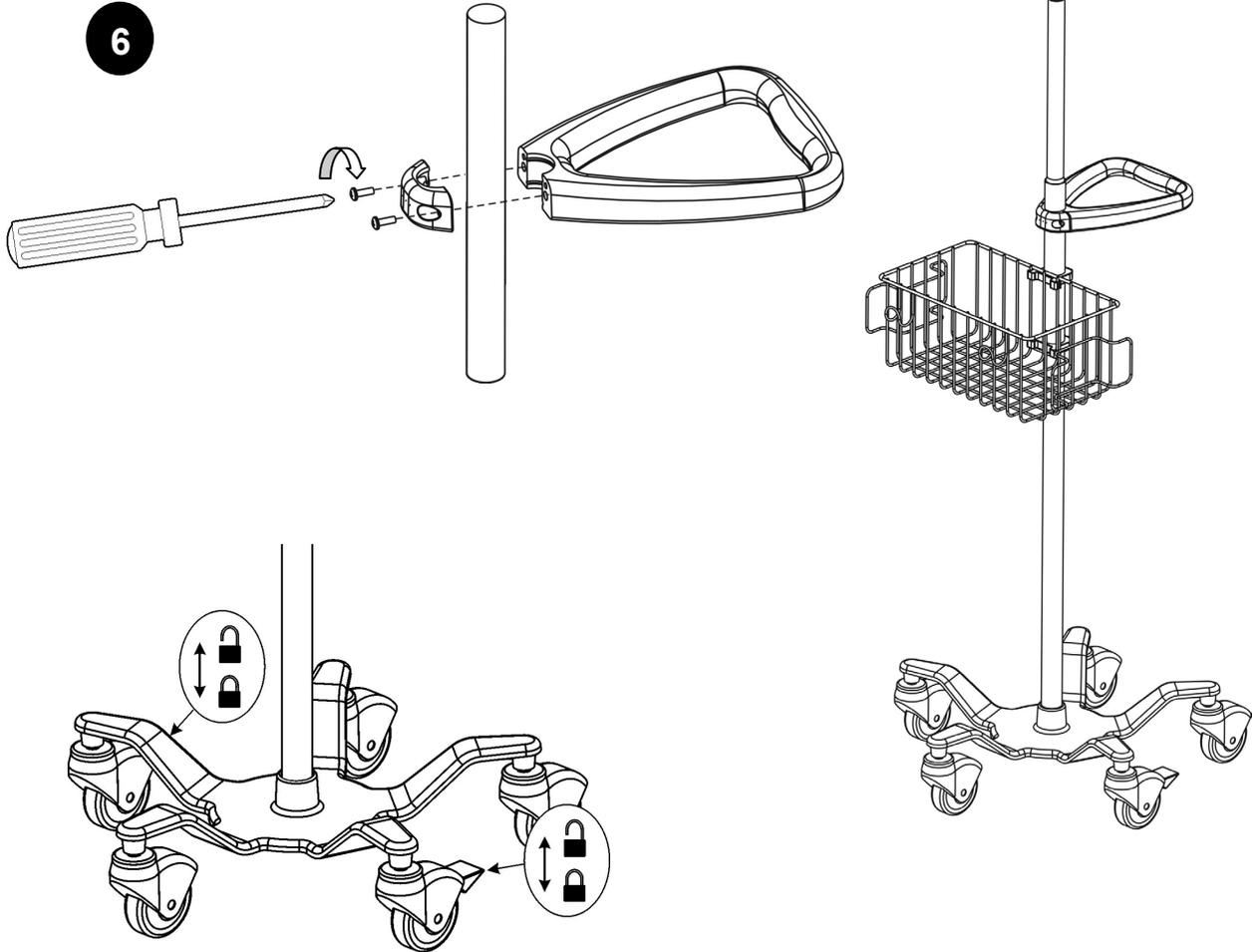
Example of devices mounted on Pole. PRC Clamps (PRC-0001-01) used for mounting both devices.
