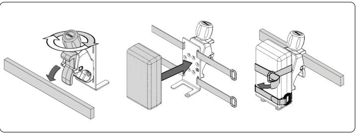
Open Clamp by turning knob counterclockwise (CCW). Position Clamp around Rail and turn Knob clockwise (CW) to tighten.
