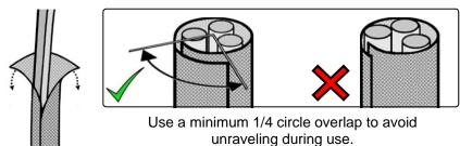
If using cable sleeves different than those provided with the arm then cut the sleeves to 30-1/2" (77.5 cm) in length and verify function within the arm prior to final product installation.
