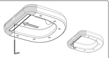
Move the arm to a level horizontal position and use a 5/32" hex wrench to increase (+) or decrease (-) the counterbalance setting.
