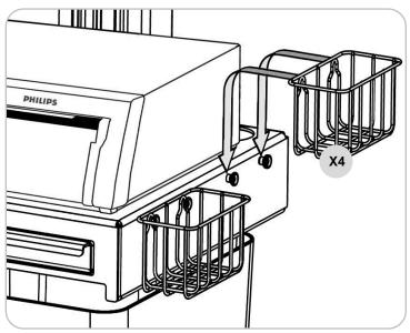
**4.** Install the (4) utility baskets by sliding them over the mounting buttons and pressing down.
