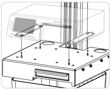
3. Lower the FM 40/50 onto the tray making sure that the (4) locating pins on the tray slide into the (4) corresponding locating holes on the mounting rails.
