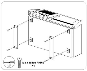
2. Secure the (2) adapter rails with (2) M3 x 18mm PHMS per rail. The locating hole on each rail must be positioned inwards.
