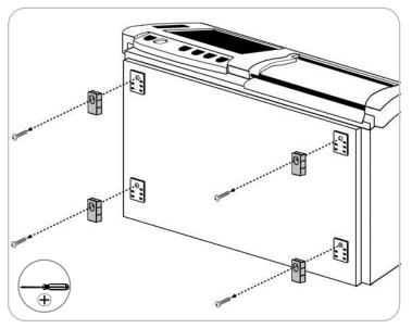
**1.** Using a Phillips screwdriver, remove the (4) screws and mounting pads
