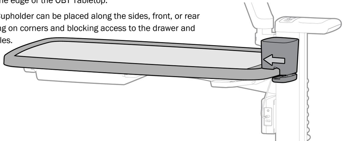
3. Once Bin/Cupholder is hooked over the edge of the Tabletop, using a Phillips Screwdriver, tighten both screws until Bin/Cupholder is secured.
