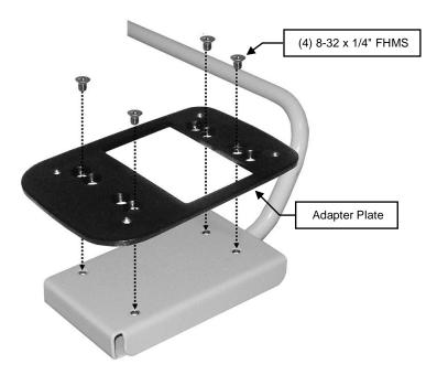
2. Install Power Cord and USB Cable in to Scanner Base per manufacturer's instructions. Fasten Base to Adapter Plate with (4) Pan Head screws included with the Adapter.
