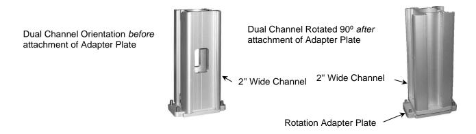
Guide Channel Slide (bottom of Column) into end of channel and move Column to desired position in channel. Using the 1/8" hex wrench provided, tighten four (4) set screws in Channel Slide to secure position of Column.
