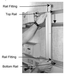
2. Secure Channel by tightening the top Rail Fitting (2) 10-32 x 3/4" OHMS & (1)10-32 x 3/4" PHMS, and the bottom Rail Fitting (2)10-32 x 3/4" PHMS
