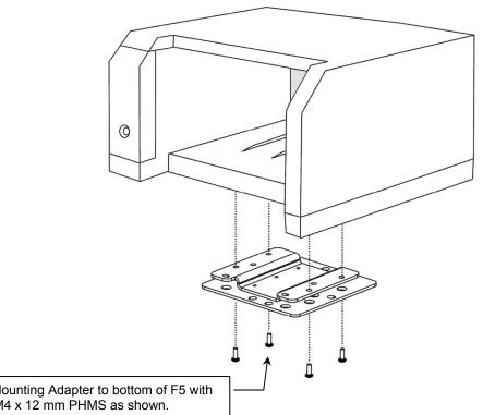
1. Fasten Mounting Adapter to bottom of F5 with four (4) M4 x 12 mm PHMS as shown.
