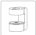
6. Position (1) 2" Nylon Washer on top of mounting arm, and (1) 2" Nylon Washer on the bottom of mounting arm. Guide Swivel Suspension Mount onto mounting arm as shown (far right).
