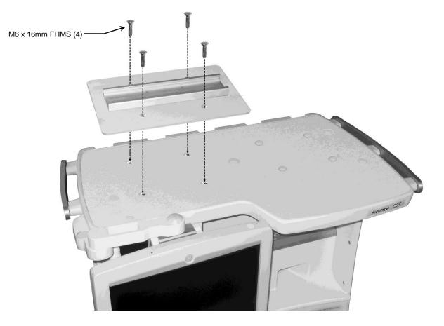
**Installation Note:** Two (2) Top Plates may be mounted side by side using both the left and right four-hole mounting patterns.
