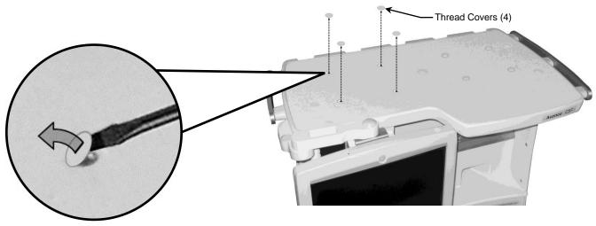
**Installation Note:** Top Plate may be mounted in two different locations: the left four-hole mounting pattern and the right four-hole mounting pattern.
