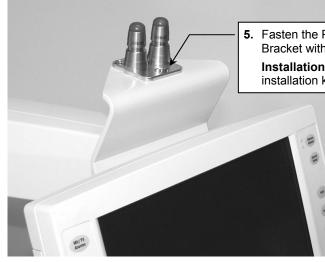
Fasten the Philips-supplied table top mount to the top of the Mounting Bracket with three (3) M6 x 8 mm FHMS.
