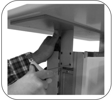
Loosen the screw that secures the Adjustable Stops (both sides of column), reposition the Adjustable Stop to the bottom surface of the Slide and re-secure.
