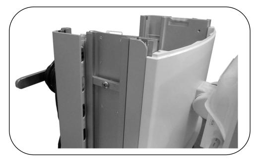
Insert Top Plate Slides into Channels on both sides of the column (orient the lip of the Top Plate to the rear of Perseus). Using 1/8" hex key, secure the four (4) set screws on each slide (minimum torque per set screw: 35 lb-ft /47.5 N\*m).
