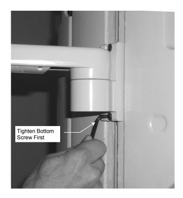
5. To adjust height of Arm in track, loosen the two (2) FHSCS, move the arm, and re-tighten screws.
