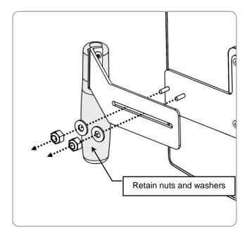
2 Install the holster onto the center plate studs using the 10-32 nuts and washers. Leave the nuts loose so holster can slide in/out. Adjust the spacing between the display and holster, and then tighten the 10-32 nuts to secure the holster.
