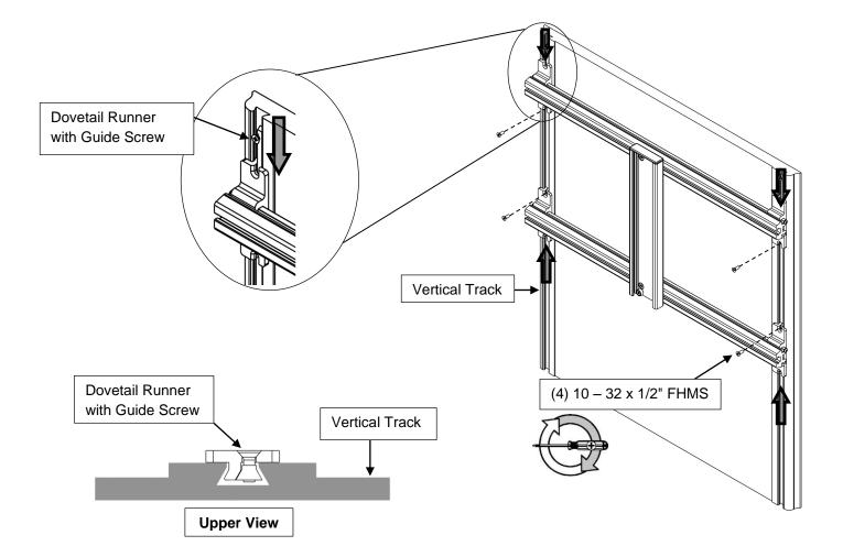
4. Using a Philips Screwdriver, alternately tighten the (8) Dovetail Runner Screws until assembly is secure. Note: use a level to check if assembly is parallel with floor
