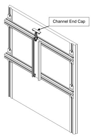
8. Using a hacksaw, cut Spanner Rail Covers to length and press Covers onto Spanner Rail until it snaps into place.
