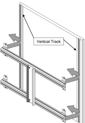
One at a time starting with the secured Face Plate, insert the (4) Dovetail Runners into the Vertical Track and position the Guide Screw in Face Plate Slot. Install (1) 10 – 32 x 1/2" FHMS on each of the Dovetail Runners.
