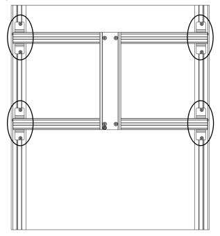
5. Using a 3/32 Hex Wrench, tighten the (2) set screws underneath the (3) remaining Face Plates to secure them to the Spanner Rail.
