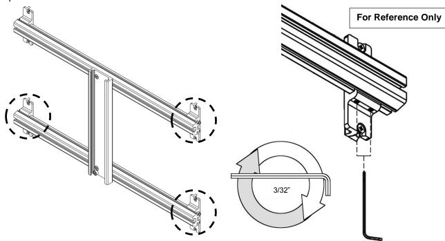
**6.** Using a Philips Screwdriver, loosen (4) 1/4 – 20 5/8" FHMS and slide channel along Spanner rail to adjust horizontal position. Alternately tighten screws to secure in position.
