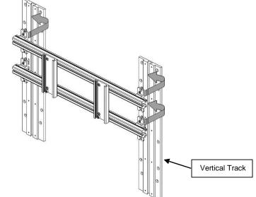
3. One at a time starting with the secured Face Plate, insert the (4) Dovetail B Runners into Vertical Track and position the Guide Screw in Face Plate slot. Install (1) 10-32 x 1/2" FHMS on each of the Dovetail B Runners. Using a Phillips Screwdriver, alternately tighten the (16) Dovetail A and B Runner screws until assembly is secure. Note: Use a level to check if assembly is parallel with floor.
