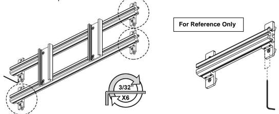
5. Using a Phillips Screwdriver, loosen (4) 1/4-20 x 5/8" FHMS per Channel and slide Channels along Spanner Rail to adjust horizontal position. Alternately tighten screws to secure in position.
