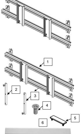
2. Position Dual Channel Mount Assembly with attached Dovetail A Runners into Vertical Track as shown. Screws must be kept loose. A second person may be needed to hold Dual Channel Mount Assembly in place.
