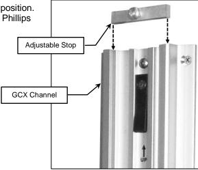
4.2 While supporting the bottom of the VHM-25 Arm, guide the Slide into the top of the Channel (right) and position it so there is a ¾" gap between the Slide and Adjustable Stop.
