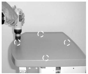
**3.** Align four (4) mounting holes in Top Plate with corresponding holes in top of machine (drilled in step 2). Fasten Top Plate to machine with four (4) M5 x 30mm Pan Head Machine Screws (PHMS)
