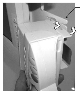
Insert four (4) tabs on the rear of the Remote Speedpoint into the slots in the Remote Bracket
