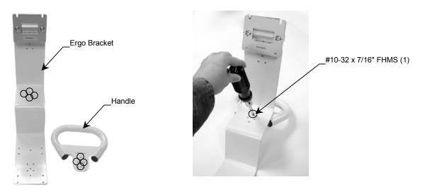
2. Attach the Ergo bracket and Handle assembly to the Roll Stand by aligning the remaining three (3) hole pattern and secure using the supplied #10-32 x 5/8" FHMS (3).
