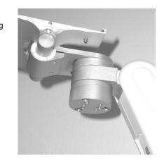
3. Align the three (3) hole pattern on the Handle, with the three (3) hole pattern on the Lower Swivel Fitting. Use the supplied #10-32 x 3/8" PHMS (3) to secure the Handle to the Lower Swivel Fitting.
