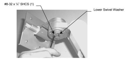
2. Take the Lower Swivel Fitting and place it over the washer, aligning the three (3) hole pattern. Secure using the supplied #10-32 x <sup>3</sup>/<sub>4</sub>" SHCS (3).
