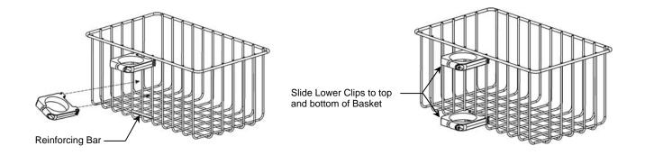
3. Slide Clips over the open end of the post. Position Basket at desired height and install two (2) #8-32 pan head machine screws (PHMS) and #8-32 hex nuts as shown below. Tighten screws until Basket does not rotate on post.
