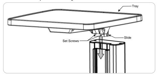
2. Using the 1/8" hex wrench (provided), tighten the two (2) set screws to secure Tray in place.
