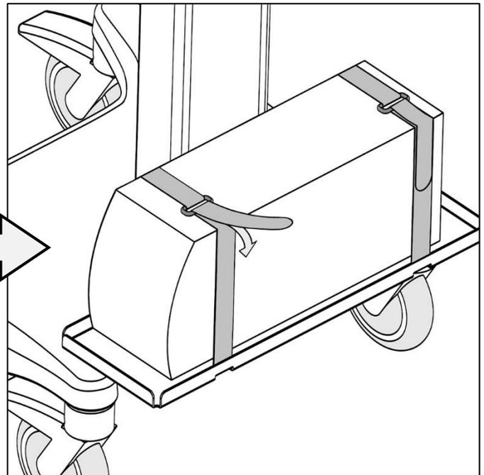
Install UPS to tray, and secure with the (2) Velcro straps.
