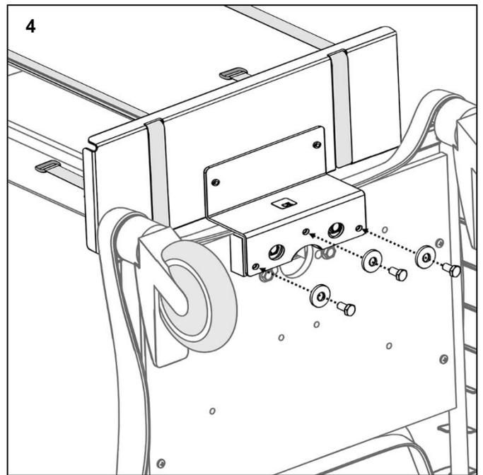
Using a 1/2" socket wrench, secure the tray assembly to the base spacer with (3) 5/16-18 x 5/8" bolts and (3) washers.
