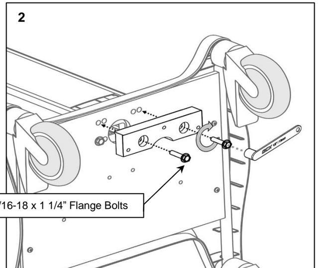
Install base spacer using (2) 5/16 x 1 1/4" flange bolts.
