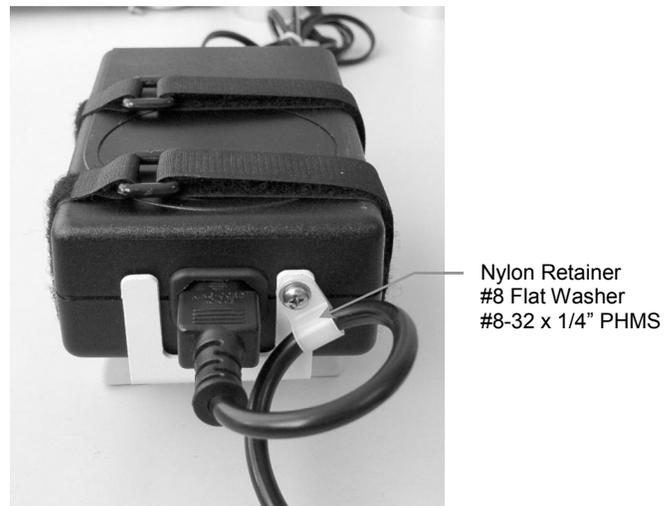
3. Fasten Clamping Blocks to Roll Stand Post with two (2) #10-32 x 9/16" PHMS (below). **Installation Note:** The power supply mounting position is determined by the application. Mounting shown below is typical for many applications but not required.
