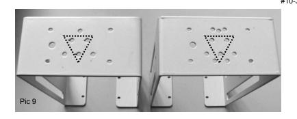
4. Mount the Module Housings in the Hangers using four (4) #6-32 x 3/8" PHMS per Housing. **Installation Note:** Use four (4) screws removed in Step 1 and four (4) screws supplied with the Installation Kit.
