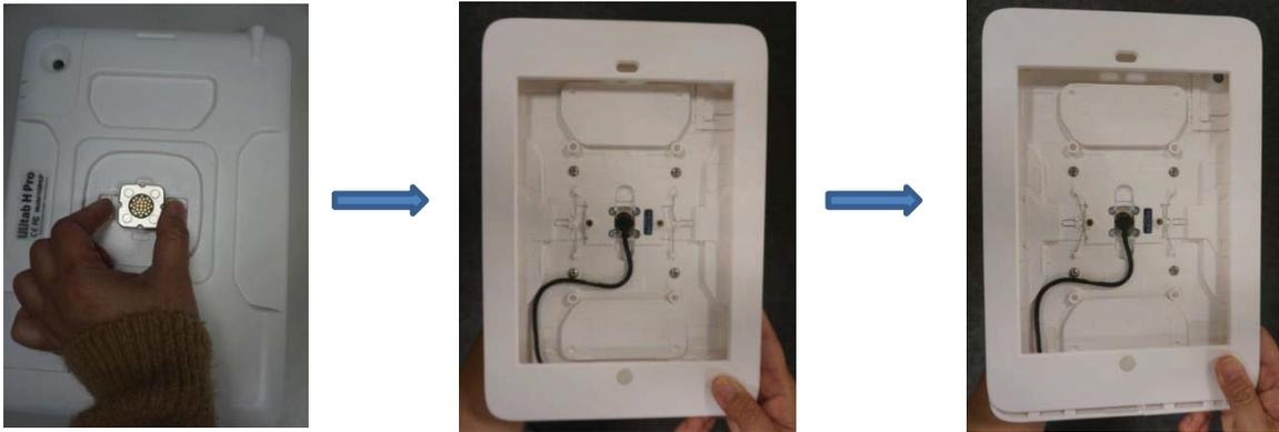
3. Before inserting your tablet, ensure the tablet charging port is on the same side as the USB Charging Cable. Lay the Mountable Tablet Enclosure face up, insert your tablet and connect the USB Charging Cable.
