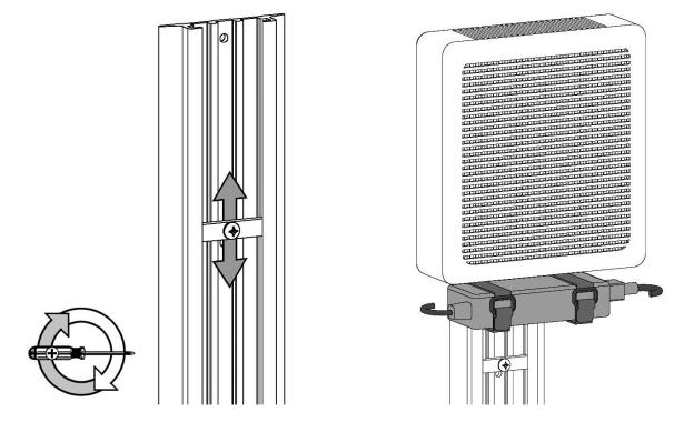
3. Using a Phillips screwdriver, tighten both screws on right side of mount to secure position.
