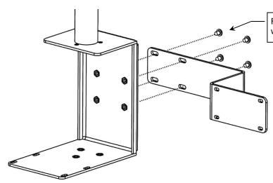
Fasten PRN-50 Bracket to rear of F5 Hanger with four (4) #10-32 x 1/4" PHMS as shown.
