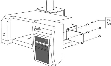
Fasten PRN-50 to Mounting Bracket with four (4) M4 x 12 mm PHMS as shown.
