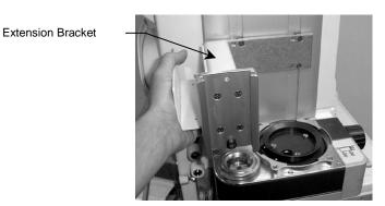
2. Insert the "B runners" as shown and secure them using the #10-32 x 5/8" PHMS with washers supplied. Position the extension bracket as desired. Tighten all eight 10-32 screws at this time, this will secure the bracket in the dovetail tracks.
