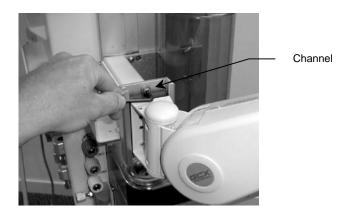
2. Install the stop screw to the rear pivot bracket on the VHM arm as shown to prevent the arm from interfering with the bellows assembly.
