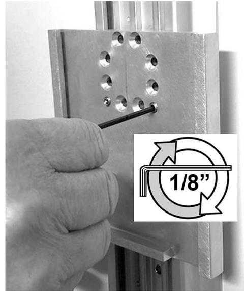
Tighten 2 set screws to secure in Channel
