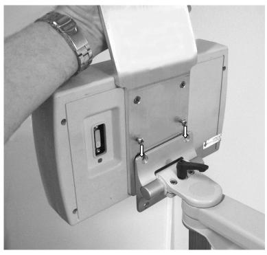
Install two (2) #10-32 x 3/8" PHMS into lower mounting holes (shown below) and tighten all four (4) mounting screws.
