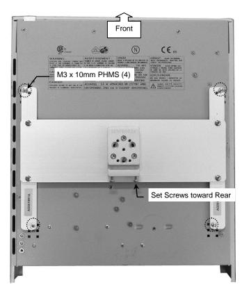
1. Slide the Mount (bottom of AGM) into the Channel and move to desired mounting position (below left).
