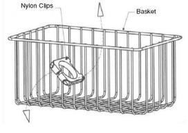
2. Slide the Clips to the top and bottom of basket. The top Clip should be touching the top horizontal wire, and the bottom Clip should be touching the lower reinforcing wire.
