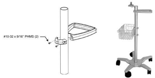
2. Position the Utility Basket beneath the Mounting Adapter Assembly (see photo above) and tighten the Basket Clips.
