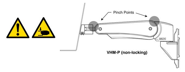
• Remove the Device only when the Arm is at the highest position. Due to the counter balance function, the Arm will naturally rise to the highest position when weight is removed. This can happen suddenly if the weight is removed at any height other than the highest point.
