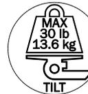
Maximum weight for mounting plate with tilt function.
