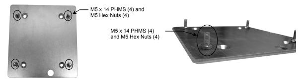
3. Re-install the mounting plate to the power supply and install Mounting Adapter using the (4) M5 Kep Nuts:
