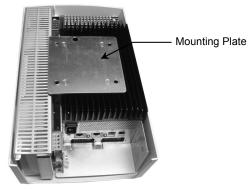
**2.** Remove the mounting, and install the (4) M5 x 14 PHMS screws using the (4) M5 Hex Nuts:
