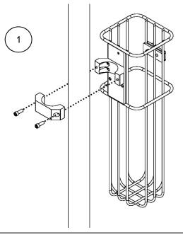
To attach the rear Clamping Block onto the E-Cylinder Basket, insert and tighten the two (2) 1/4-20 x 3/4" (SHCS) as shown.
