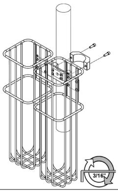
To attach the rear Clamping Block onto the Crossmember, insert and tighten the two (2)  $1/4-20 \times 3/4$ " (PHMS) as shown.
