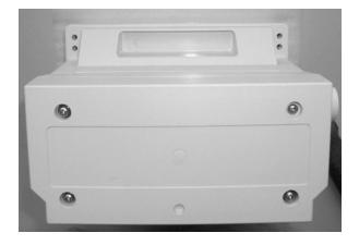
2. Slide Mounting Pan/Adapter assembly over rear of monitor, aligning two (2) mounting tabs with handle-mounting holes. Reattach handle with screws removed in Step 1.
